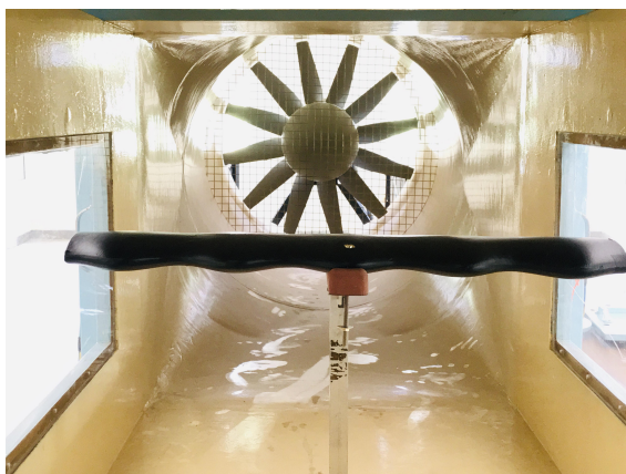
Figure 14: Wing model undergoing testing in Wind Tunnel
