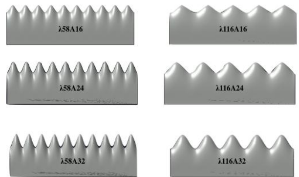
Figure 4: Tubercle Models of various Wavelengths and Amplitudes
