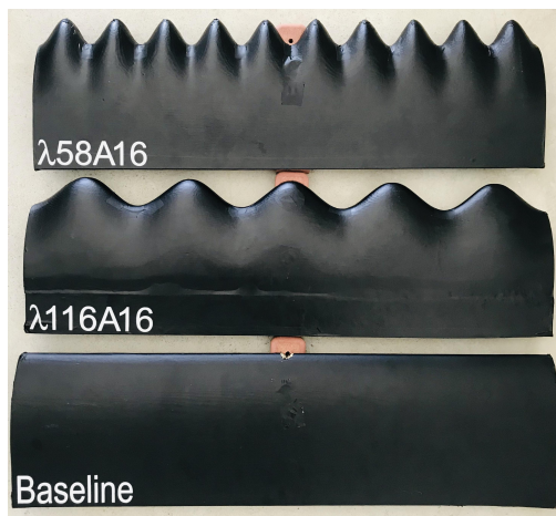
Figure 13: Fabricated wing models
