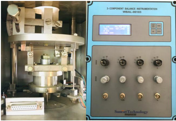
Figure 12: 3-Component balance setup
