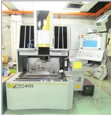
Figure 1. AG40L Sodick electrical discharge machine
