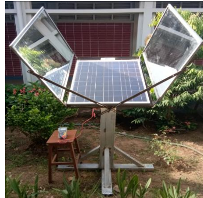
Figure 7. A solar PV panel using mirror as reflectors
