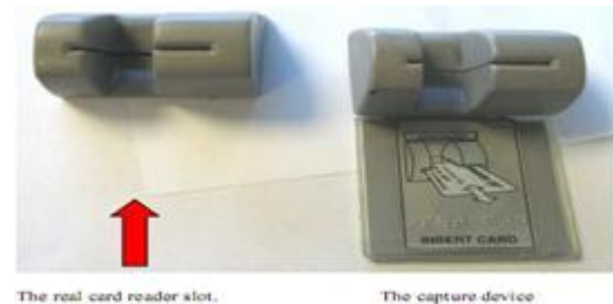
Figure 1 ATM Skimming Device. (Krebs, 2010)
