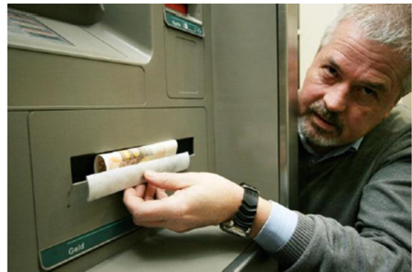
Figure. 5 Cash is trapped by the false withdrawal shutter. Source: (Agarwal, 2010)
