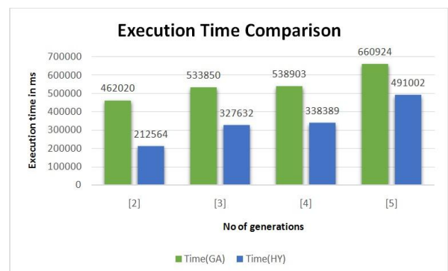
Fig. 7: Graph showing Execution Time values of Genetic Algorithm and Hybrid approach corresponding to number of Generations.
