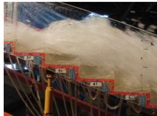
Figure 6b. Slope=12°, height of end sill=15mm and thickness=5mm
