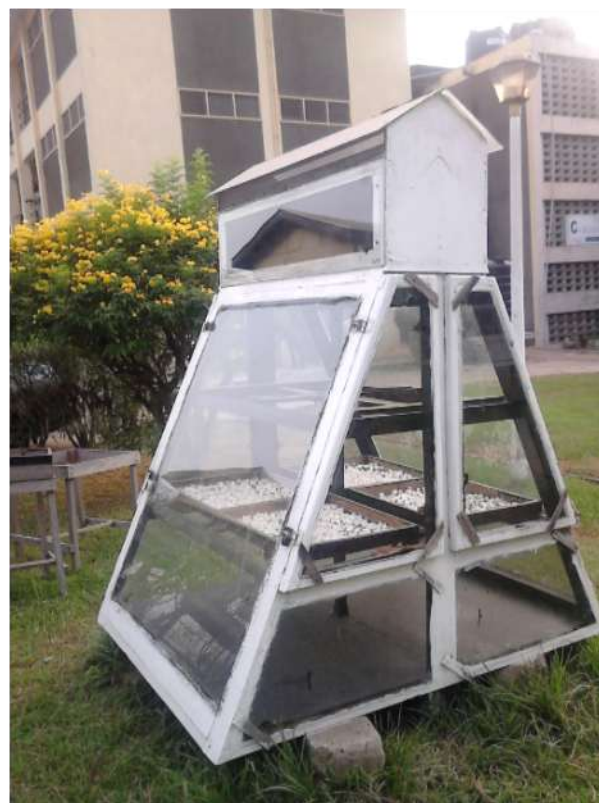
Figure 4 Pictorial view of a solar tent dryer equipped with a solar chimney
