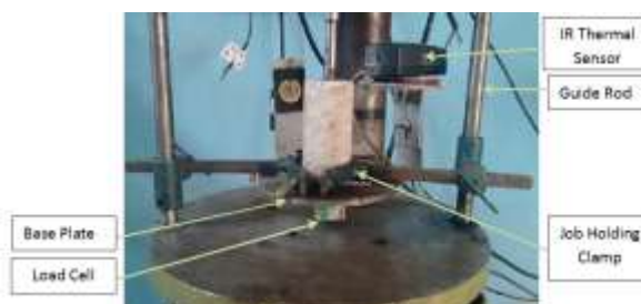
Figure 7: Arrangement showing guide rod with job holding clamp
