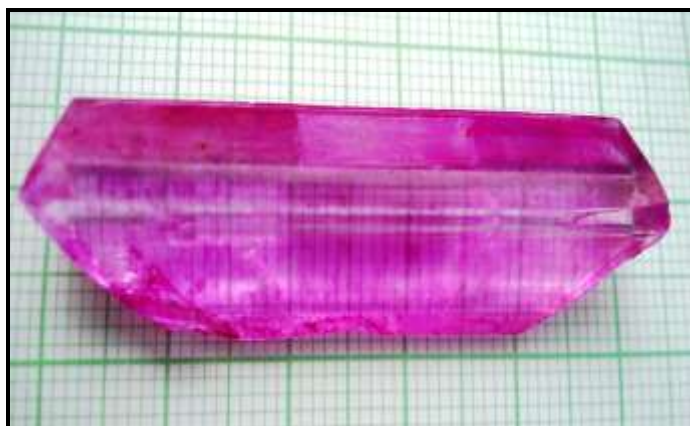
Figure 2. Grown RBLATU crystal
