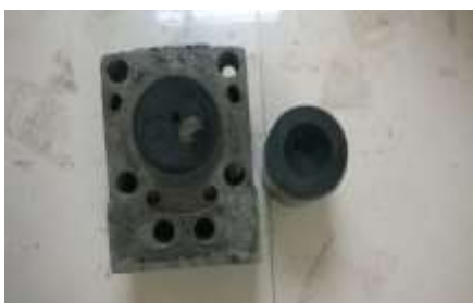
Figure 2: UnCoated piston crown and Cylinder head
