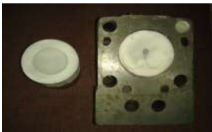
Figure 1: Coated piston crown and Cylinder head
