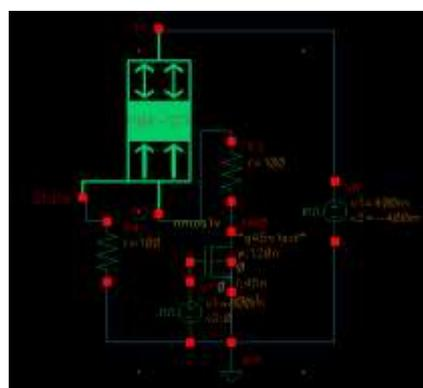
Figure 5(a) : Schematic of 1T-1MTJ cell (PMA)
