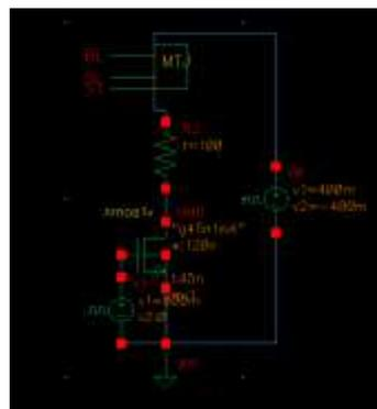
Figure 4(a) : Schematic of 1T-1MTJ cell (IPS)
