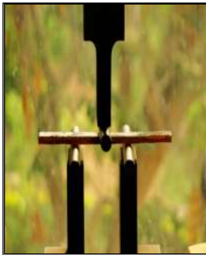
Figure 3.1–Test Specimen undergoing flexural test
