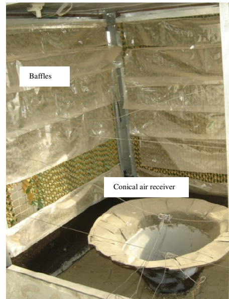
Figure 4 Arrangement of conical cool air receiver and baffles on cooler grill
