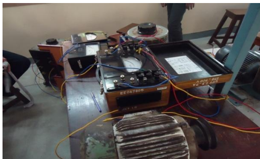
Figure 2 Snap shot of open and short circuit test
