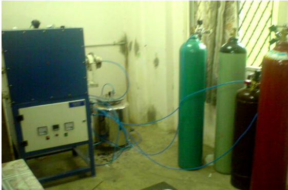
Figure 2. Experimental setup of CVD system
