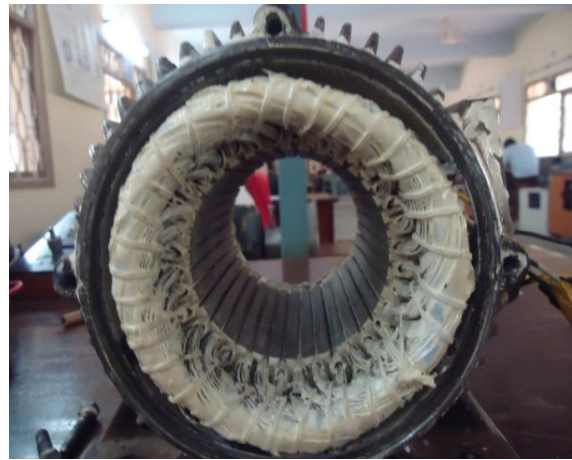
Figure 1 Nanocomposite filled enamel coated induction motor
